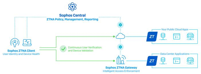
Sophos ZTNA is also unique in that it integrates tightly with both Sophos Firewall and Sophos Intercept X endpoints. This allows for taking advantage of Synchronized Security and Security Heartbeat to share device health between the firewall, device, ZTNA, and Sophos Central to automatically respond to threats or non-compliant devices. Automatically limit access and contain compromised systems until they are cleaned up.
