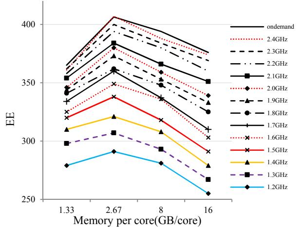
Fig.20. Energy efficiency with different memory per core and CPU Frequency on #4 server.
