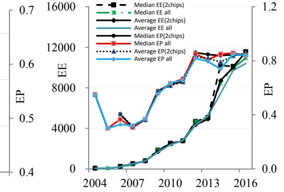
Fig.15. Comparison of EP and EE of single node servers with 2 chips to all servers.
