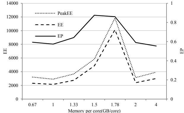
Fig. 17. EP and EE at different memory per core configuration.
