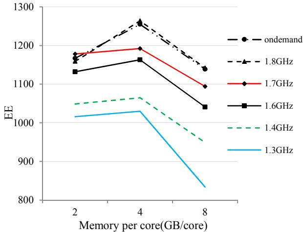
Fig.19. Energy efficiency with different memory per core and CPU Frequency on #2 server.
