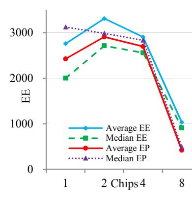
Fig. 14. EP and EE of single node servers.
