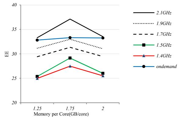
Fig.18. Energy efficiency with different memory per core and CPU Frequency on #1 server.
