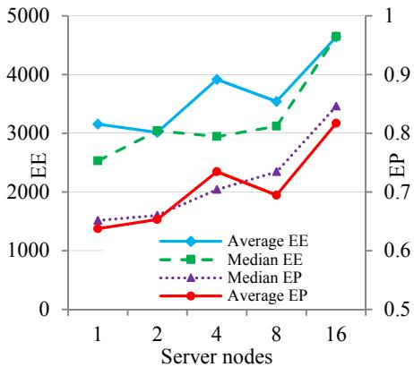
Fig. 13 EP and EE improve with server nodes.
